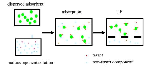
Ultrafiltration combined with process of sorption
